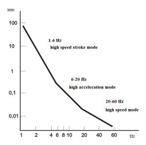
1-picture. The graph of the dependence of Jane on the vertical vibration, which is limited for convenience to passengers [2]. In the work of the author below, the empirical equation of dependence on frequency, vibration amplitude of discomfort (discomfort) is defined:
