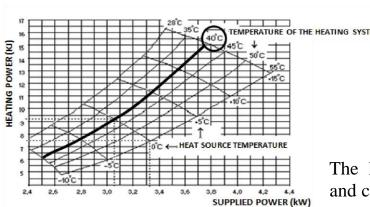
Figure 4. Diagram for determining COP.
