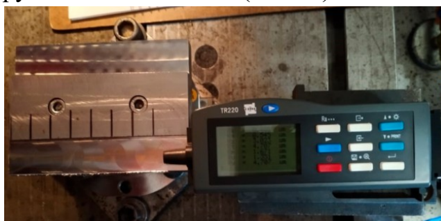
5-rasm. Sirt g'adir-budurligi o'lchovi (TIME Model: TR220)
