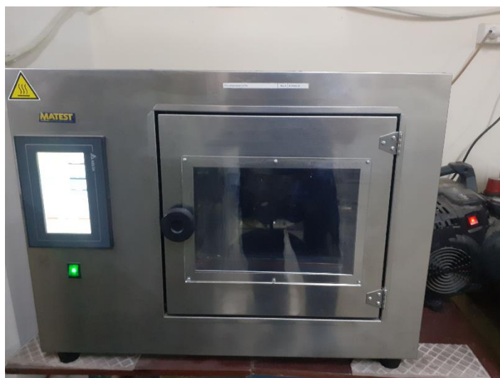
Figure 1. Short-term aging process of conventional 50/70 penetration grade bitumen and hydrated lime-modified bitumen using the RTFOT apparatus
