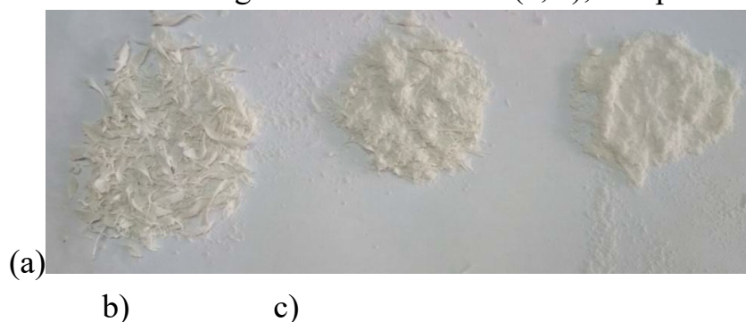
Figure 7. Effect of tool wear on chip formation
