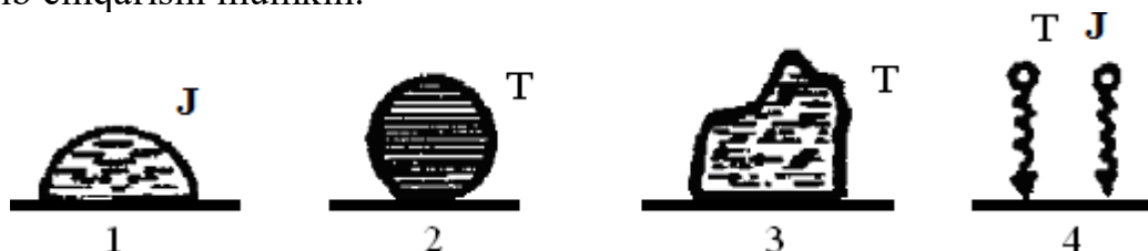
1- rasm. Yuzada radioaktiv ifloslanish: J-suyuq va T-qattiq holat.
