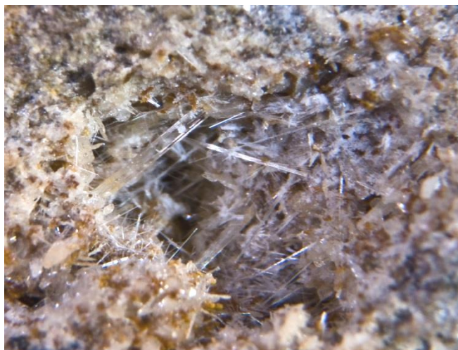
Figure 1. Microignacious structure of wollastonite (magnified 1700 times).
