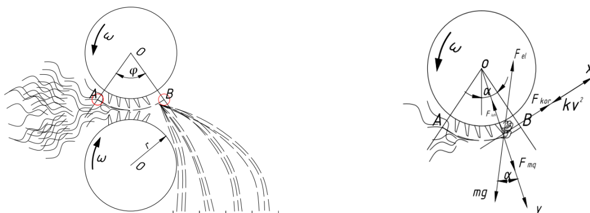
2-picture. Scheme of the effect of the pinching roller on wool fibers affecting the separation of wool fibers
