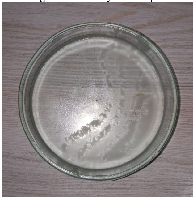
Figure 3. Na-CMC sample degraded under open-air conditions In the second sample, no changes were observed. However, when the second sample was heated in a dry air oven, degradation occurred.
