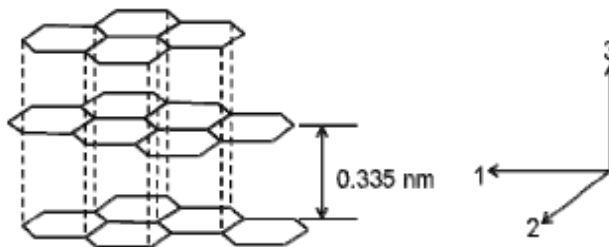
Figure 1. Structure of graphitic crystals and crystal directions.
