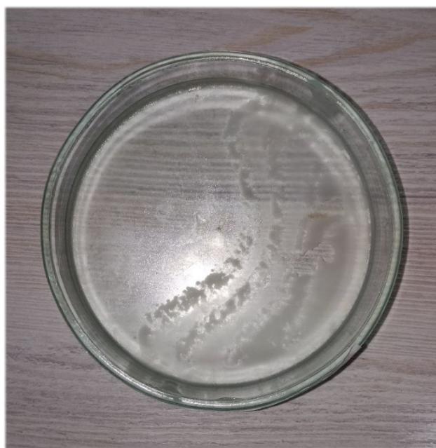
Figure 3. Na-CMC sample degraded under open-air conditions
