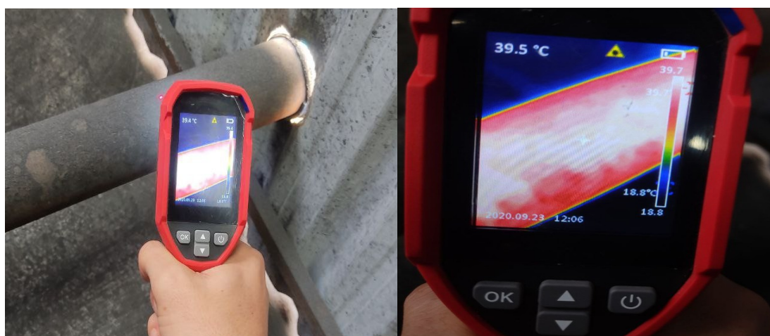
Figure 1. Measuring temperature in pipes using an infrared thermal camera.
